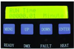
Note: Once the machine is started, the cumulative running time will be displayed automatically, including the actual spraying time but excluding the standby and warm-up time. The cumulative time is maximum 60000.00 minutes and accurate to a second. If the cumulative time exceeds 60,000 minutes, the system will automatically clear it and re-calculate the time, as shown below:
