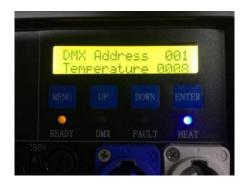
When the machine is working, the warm-up function will be enabled automatically, and the DMX address and real-time core temperature will be shown. If the temperature sensor is abnormal, the FAULT indicator will flash, and the following interface will pop up.
