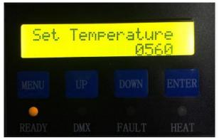
Press UP or DOWN to set the temperature between 560°C and 620°C. Then press ENTER or MENU to go back to the working status interface.
