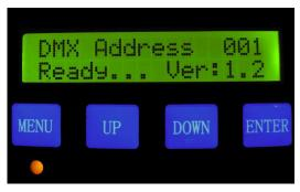
Note: The DMX address saved last time and "Ready For Work..." will be shown on the standby interface. The user can enable warm-up via the DMX stage controller or press MENU to enter the working status interface.
