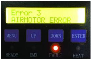
If the above interface pops up, immediately shut down the machine and return it to the factory for repair.
