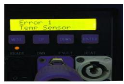
If the temperature sensor is in the normal status, warm-up will be started. The HEAT indicator will flash in the warm-up process. After warm-up, the HEAT indicator will be OFF.
