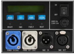
4.1.1 LCD information display area: displaying the operation menus and equipment running status.
