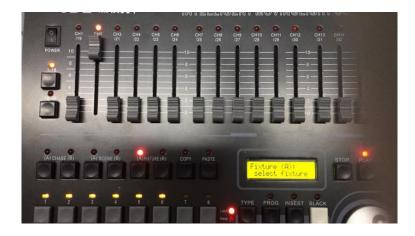
6.8 When the core temperature reaches the set value, push the first push rod of the controller to start spraying according to the firework height. The firework height depends on the push rod data: 10-19 as the first gear, 20-29 as the second gear, 30-39 as the third gear, 40-49 as the fourth gear, 50-59 as the fifth gear, 60-69 as the sixth gear, 70-79 as the seventh gear, 80-89 as the eighth gear, 90-99 as the ninth gear, and 100 and more as the tenth gear.
