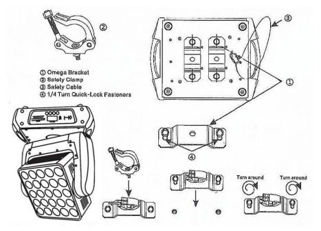
Regardless of the rigging option you choose for our Matrix moving head, always be sure to secure your fixture with a safety cable. The fixture provides a built-in rigging point for a safety cable on the hanging bracket as illustrated above. Be sure to only use the designated rigging point for the safety cable and never secure a safety cable to a carrying handle.
