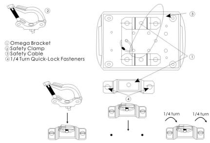
Regardless of the rigging option you choose for your LED moving head, always be sure to secure your fixture with a safety cable. The fixture providers a built-in rigging point for
