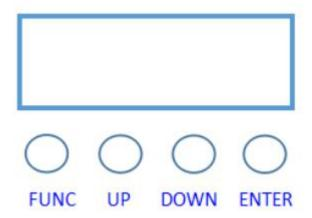
Operating instructions: Press the function key FUNC to cycle out 8 different function effects (refer to the function table), UP and DOWN adjust the value size, ENTER to confirm and save.
