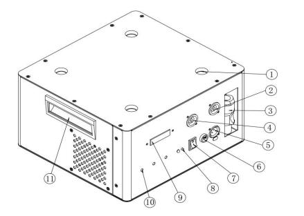
1. spark machine place2. Charging or4. Charging input interface5. DMX out7. switch8. ID code but
